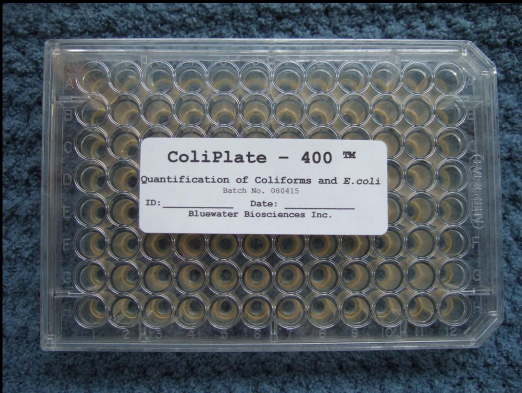
Water samples poured into 96-well colipates
